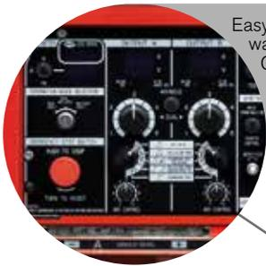
Easy operator interface with 3 way switching in either Welding, Generating or simultaneous modes. Emergency stop and key lockable operation modes.
