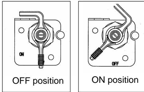
When turning the switch to OFF, the engine electric circuit does not activate due to no battery power.
