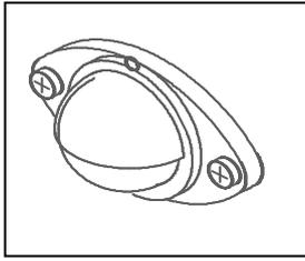
Panel light turns ON to illuminate the panel, when turning the switch (by the light) to ON.
