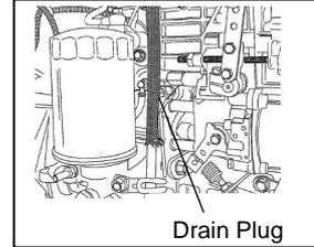
5 Remove the Sub Tank Stay and drain coolant in the Sub Tank.
