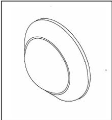
The lamp indicates whether or not the equipment is generating electricity when the engine is running.
