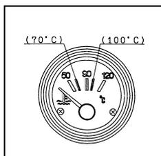
Water Temperature Gauge displays the temperature of engine coolant. Normal temperature may vary depending on the environment, but it should be between 75°C and 100°C.
