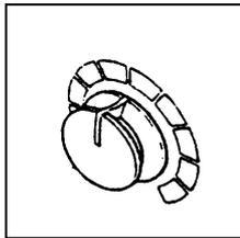
The dial adjusts generator output voltage.
