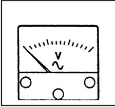
Voltage Meter displays the output voltage (Phase to Phase) from the generator.
