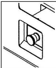
This button is used to stop the engine in emergency.
