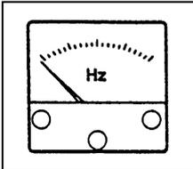
Frequency meter will display the frequency of the generator.
