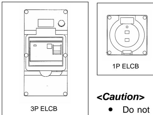
Each receptacle, 3-Phase and 1-Phase is incorporated with ELCB respectively. When current leak occurs, it trips to stop power transmission to load.
