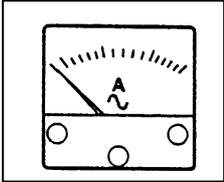
Ampere Meter displays the output current (Phase) from the generator.
