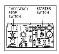
② Turn the Emergency Stop Switch to arrow mark (clockwise) to release the feature.
