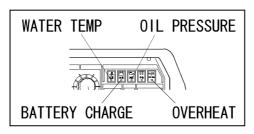
Under normal condition, when the starter switch changes from STOP to RUN, all the lamps of BATTERY CHARGING, OIL PRESSURE and Hz/OVERHEAT turn ON.
