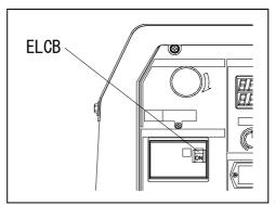
■ The Circuit Breaker has activated due to overload
