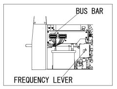
④ Turn the selector switch and the metal bus bars to the other frequency as per the drawing.
