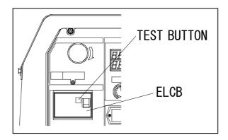
In the event you cannot complete all steps in the above procedure to the end, the device is out of order. Consult with our authorized distributor or our engineering section to repair.
