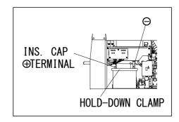
Reinstall a new battery in the reverse order.(Install always the cable to the positive (+) post in the new battery first.)
